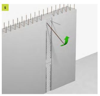
Bend the reinforcement bars back to the planned position using a rebending pipe with an inner diameter that is only slightly larger than the bar diameter.
