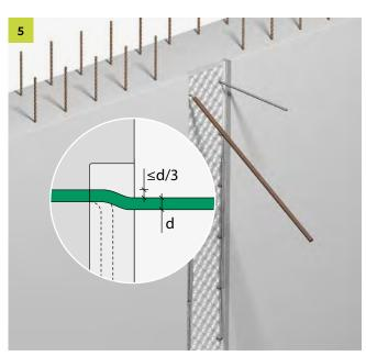
The permissible crimping value and other recommendations with regard to rebending can be found in the DBV bulletin entitled "Rückbiegen von Betonstahl und Anforderungen an Verwahrkästen" ["Rebending reinforcing steel and requirements for casing"].
