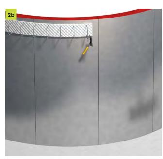
Carefully bend the casing to the correct shape so that it conforms to the shape of the formwork. Fasten it as described in step 1.
