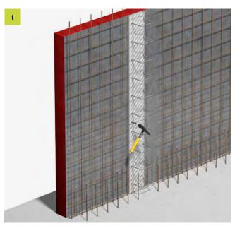
Fasten the FERBOX  $^{\! \circ}$  rebend connection in the correct position on the formwork:
