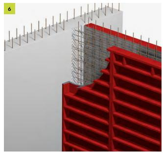
Once all the bars have been fully bent back to the planned position, erect the formwork for the second concreted section and concrete it.
