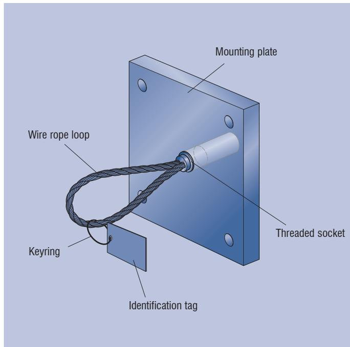
The system components of the PFEIFER LSP Lifting Loop are:
