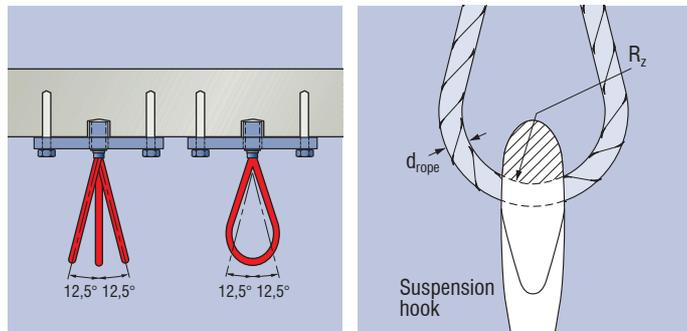
PFEIFER LSP lifting loops are for subsequent fitting in the ceiling undersides of lift shafts. They are only for temporary suspension of lift cabins or other objects during installation or maintenance work, always without transporting people and never to protect against falling. In selecting the attachment device, the corner radii  $R_z$  as in Table 2 must be observed.
