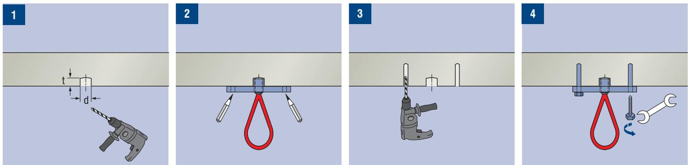
**Caution:** Incorrect fixing of the dowels will result in a reduced load-bearing capacity. This causes a hazard to life and limb. The dowel system used must be dimensioned and fitted as documented by the manufacturer concerned.
