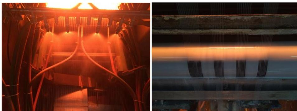
FIGURE 2: PRODUCTION PROCESS OF THE CEM-FIL® AR GLASS FIBERS (LEFT: PICTURE A; RIGHT: PICTURE B)
