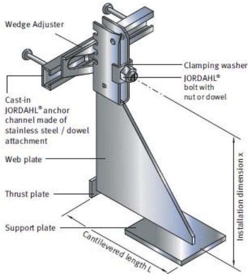
Figure 1: Brickwork support bracket with cast-in anchor channel
