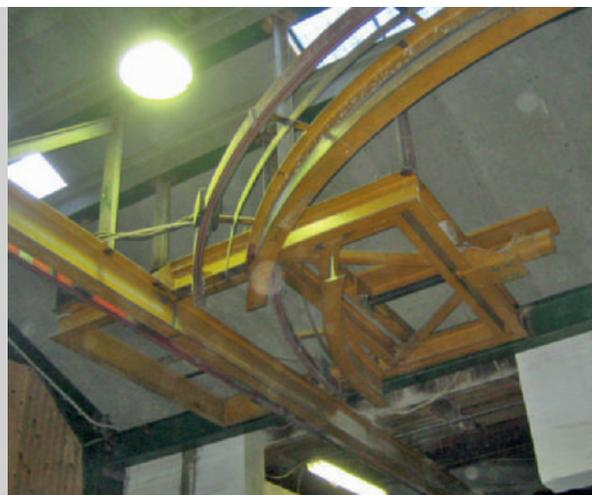
Switch-track for mono-trans concrete travelling bucket.
