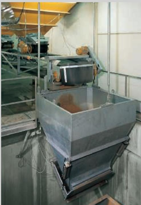
Combined weighing system with lattice weigh belt and weigh hopper.
