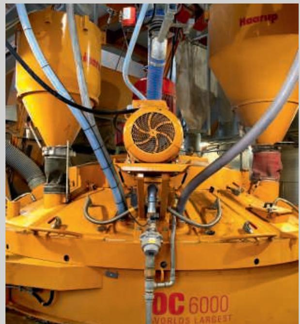
Water pump for intermediate cleaning of the mixer.
