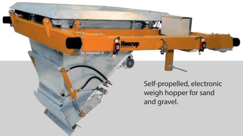
Self-propelled, electronic weigh hopper for sand and gravel.
