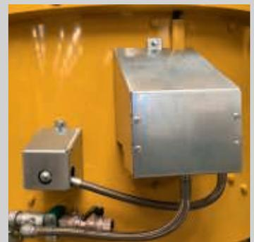
The water nozzles of the face-mix mixer can also be equipped with specially developed air/water valves for efficient cleaning of the nozzles with air.
