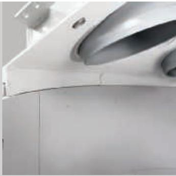
The mixer cover is smooth on the inside to reduce the build-up of materials.
