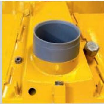
The suspension arms of the gearbox are designed for inlets so that access to service and cleaning is the best possible.
