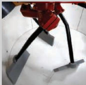
Special shovels with a selfcleaning effect which minimise the build-up of materials on the surface.
