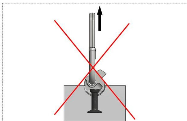
**If the shackle remains in the position showed above, the lifting of the concrete unit is not allowed**
