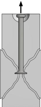
For vertical plates, the possibility that a horizontal break out can occur must be taken into account. The vertical reinforcement present has no effect on the anchoring force here either. The situation in the figure will become very critical if the thickness of the element is less than half the thickness of the T-slot anchor selected. In this situation, additional consultation with Terwa is necessary.
