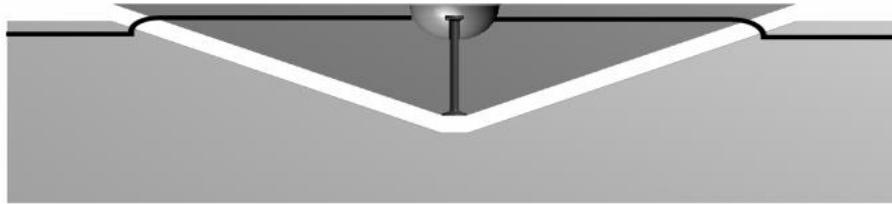
The anchoring force of the T-slot anchor is highest when the T-slot anchor is placed at a distance to the edge 3 times greater than the built-in depth so that a complete break-out cone can be created. If it is not possible to have an edge distance of 3 times the built-in depth in all directions, better anchoring must be obtained with the aid of a longer T-slot anchor.
