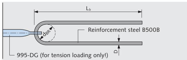
Additional reinforcement (not in scope of delivery)
