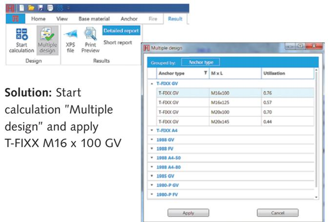
**Solution:** Start calculation "Multiple design" and apply T-FIXX M16 x 100 GV
