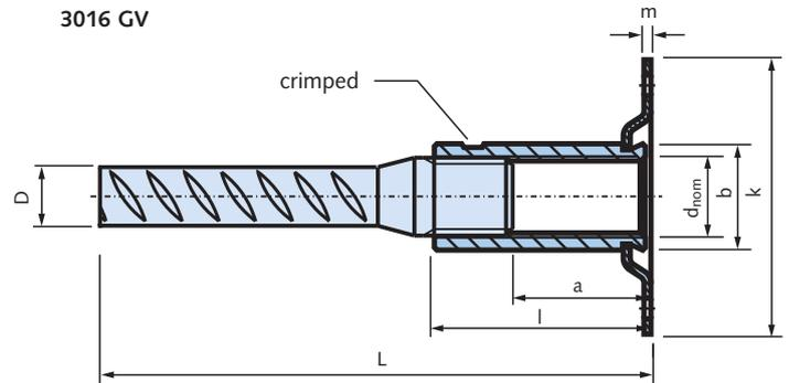
The sleeve is zinc galvanized (GV), the internal thread is metric ISO.
