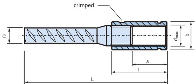
The sleeve has a metric ISO thread and is made of stainless steel (strength class A4-80).
