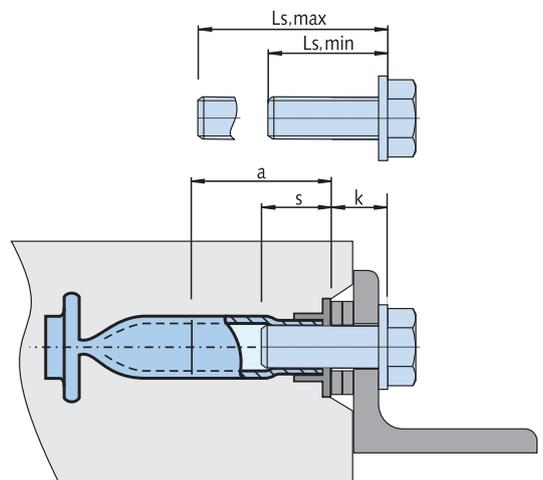
Fixing T-FIXX M12×70 to formwork with plastic nailing plate
